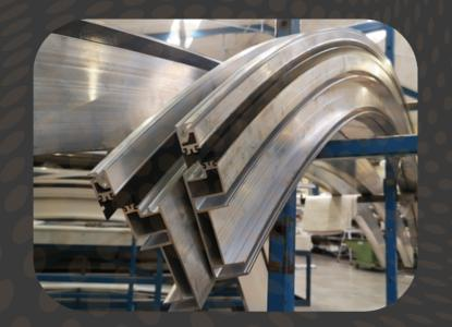
e.g. profile for facade construction that already includes a thermal break
